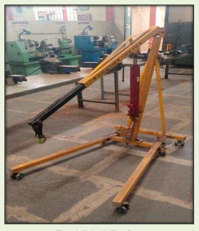
Figure 3: Hydraulic Floor Crane
